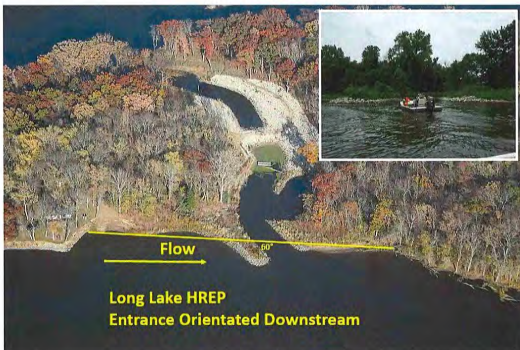
Figure 5. Example of the bedload deflector that will be utilized for the Sam Gordy's restoration project. The bedload deflector is modeled after the Long Lake habitat project near Trempealeau, WI. This structure has functioned very well for many years.
