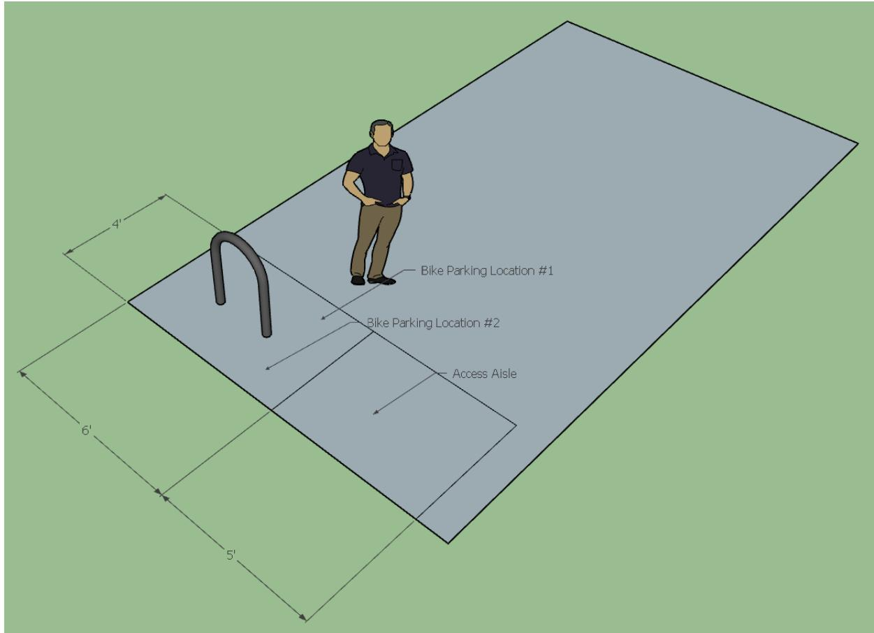
*Sample Diagram of correctly installed facility providing two bicycle parking spaces in a 12'x22' single-stall garage*
